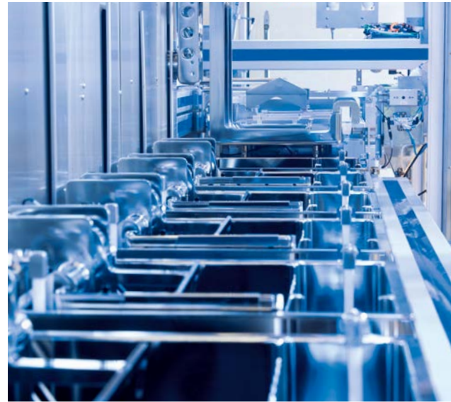
Wet Processing System for Cleaning and Coating of Eye Glass Lenses
