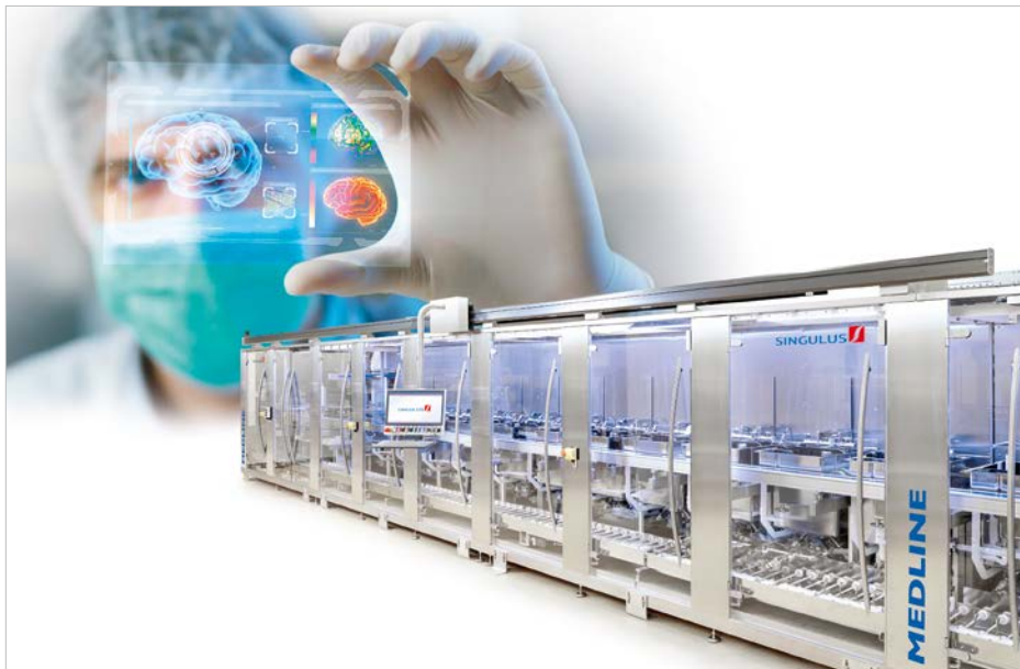
MEDLINE – Production system for cleaning and coating of contact lenses. The MEDLINE Clean cleans the contact lenses of material residues and coats the lenses in a further process step.
