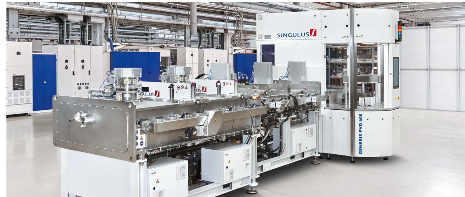
GENERIS PVD 600 Sputtering System for the application of layers as part of transmission units in mobile communication technology.
