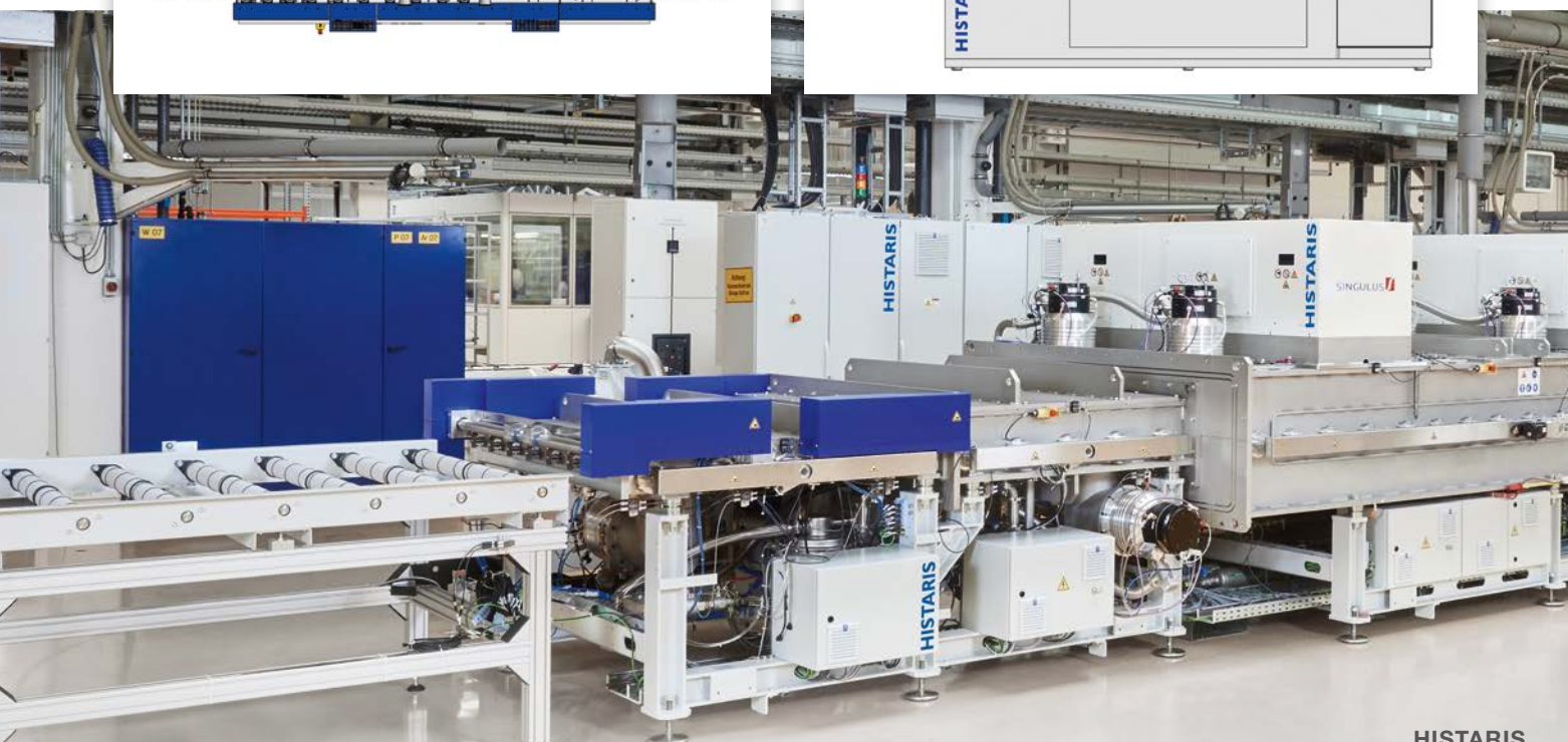
HISTARIS Flexible inline sputtering system with modular chamber arrangement for different applications
