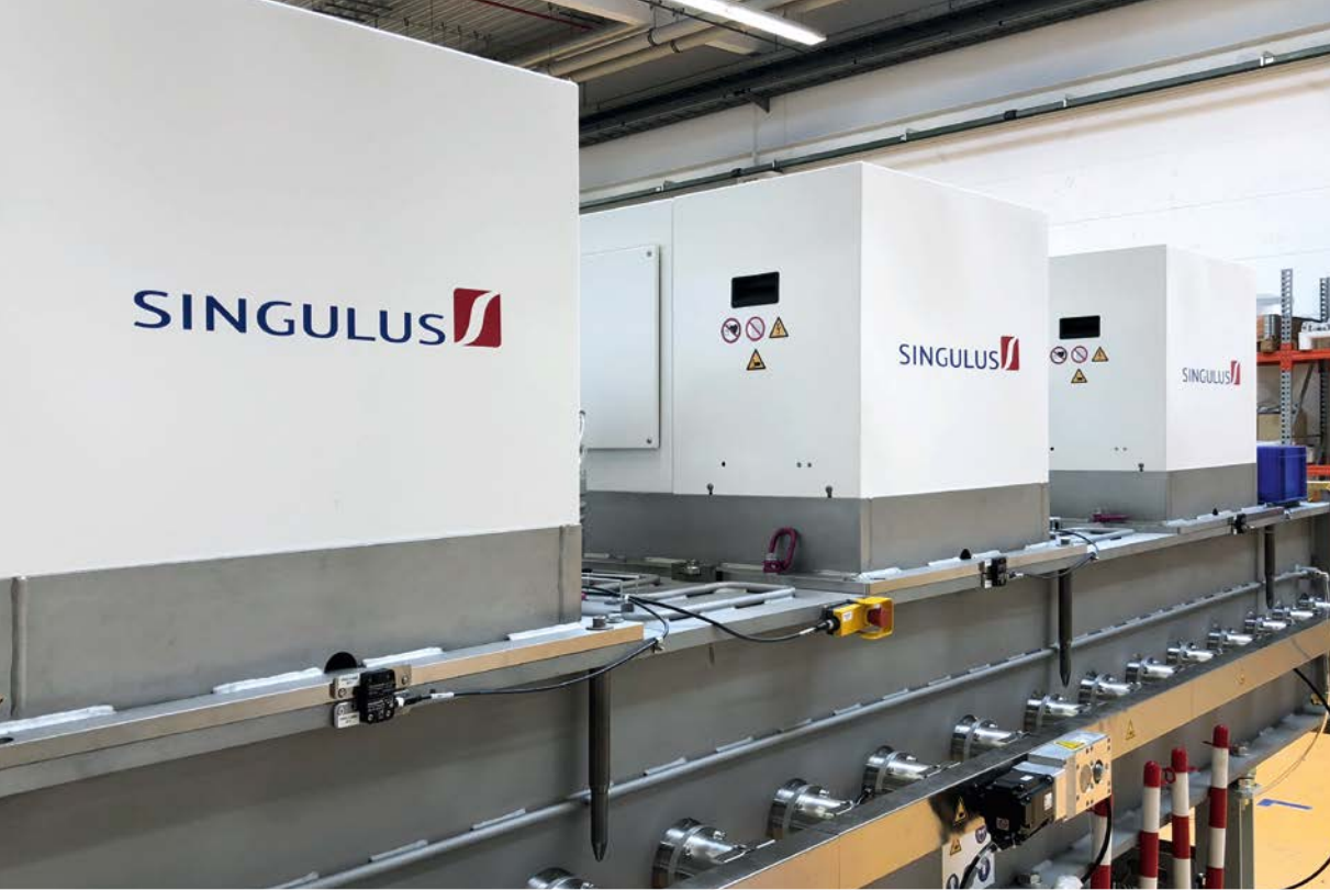
Horizontal cathode arrangement with usage of rotatable cylindrical magnetron for highest utilization of target material
