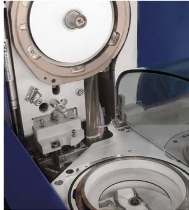
Single substrate sputtering system
