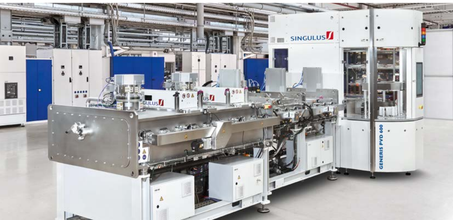
GENERIS PVD 600 sputtering system with automatic substrate loading e.g. for mobile applications
