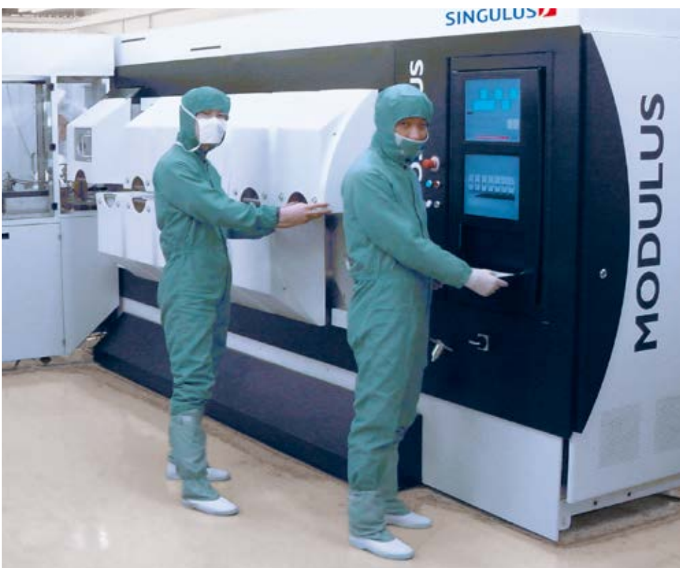
Multi-cathode inline sputtering system
