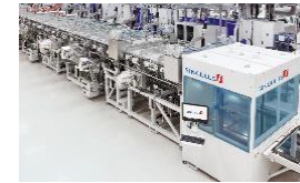
CSS Close Spaced Sublimation (CSS) for the Production of e.g. CdTe Solar Modules
