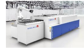
GENERIS PET System for Edge Passivation
