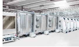
VISTARIS Inline Sputtering System with Vertical Substrate Transport
