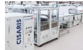
CISARIS Selenization/Sulphurization with High-End Rapid Thermal Process (RTP)
