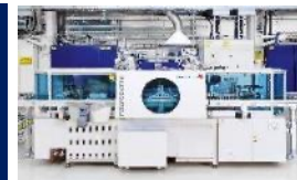
POLYCOATER Inline sputtering system
