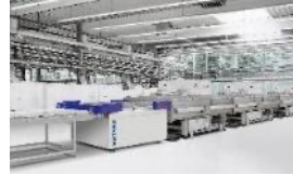
HISTARIS Inline Sputtering System with Horizontal Substrate Transport for Glass Applications
