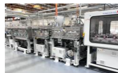
EVARIS Inline Evaporation System Horizontal Transport (Perovskite Application)
